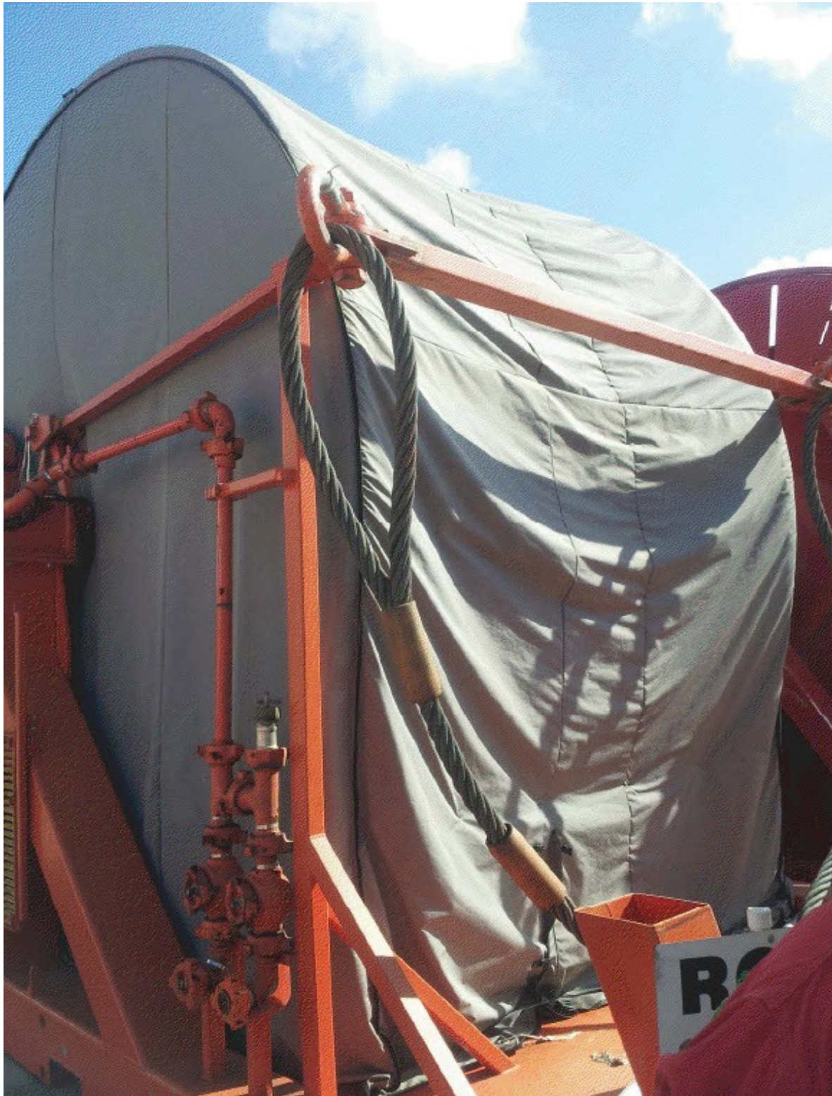
Envelop Reel Cover After Being Installed During Hurricane Isaac
