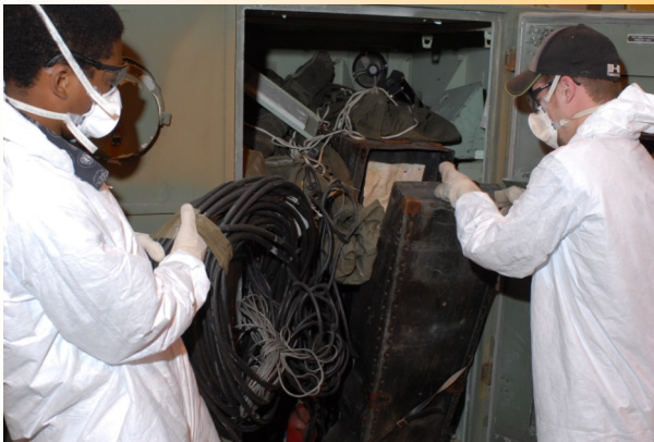
Tobyhanna DS2 Contractors Yardley Jean-Baptiste (left) and Cody Highhouse remove outdated electronic equipment and components from shelters as part of the De-Mil process. This equipment is then palletized and shipped to the Local DRMO for destruction.
