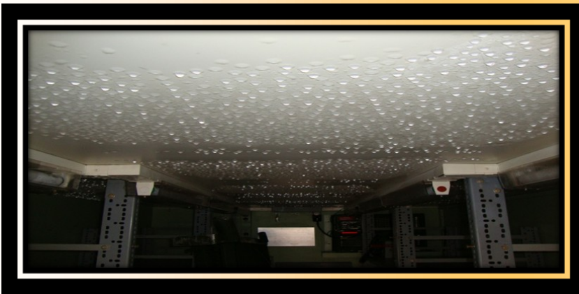
Water intrusion within CECOM shelters stored in LBE resulted in shelter deterioration and component damage
