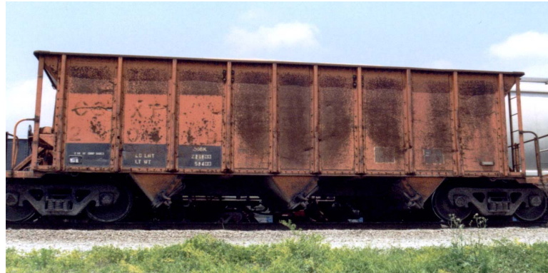
Figure 1-1. Corroded Car of Freight Train
