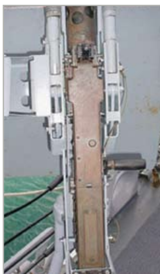
.50-caliber gun following no maintenance during two weeks in rough seas aboard the USS RUSSELL while training in the Pacific when covered with Envelop Protective Covers.
