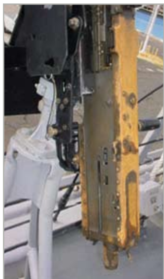
.50-caliber gun following no maintenance during two weeks in rough seas aboard the USS RUSSELL while training in the Pacific when covered with a traditional tarp.
