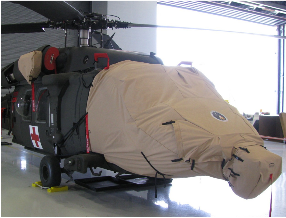
HH-60M Full Cockpit/Nose & FLIR– Part Number 122047, External Rescue Hoist– Part Number 122044, UH-60 Pitot Tube– Part Number 122042, HH-60M ECS Intake Plug 122048
