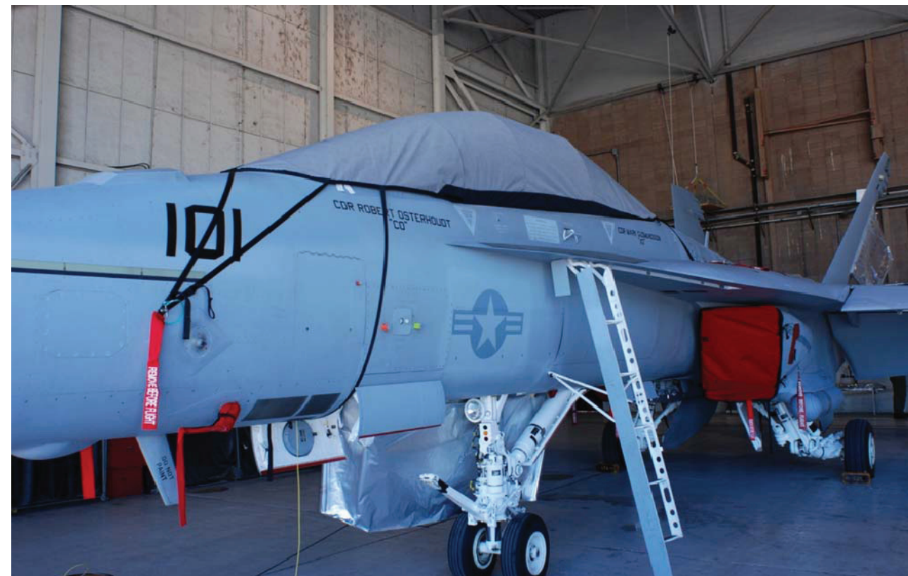
F-18F-E/A-18G Canopy- Part Number 122058, F-18E/F-E/A-18G Left Intake- Part Number 122066, F-18E/F-E/A-18G Right Intake-Part Number 122067
