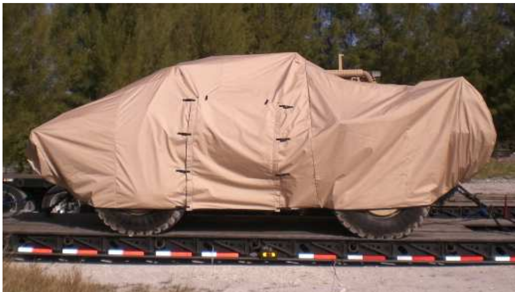
Installed ASV M1117 Gunship Cover. Part Number 123166
