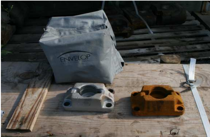
Cast iron after 2 months of testing with an oil company near the Gulf of Mexico. Proving a 90% reduction in corrosion when using ENVELOP covers.
