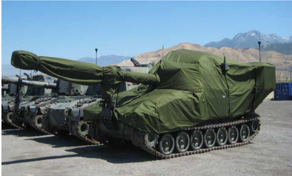
Installed Paladin M109A2 Cover Set.
