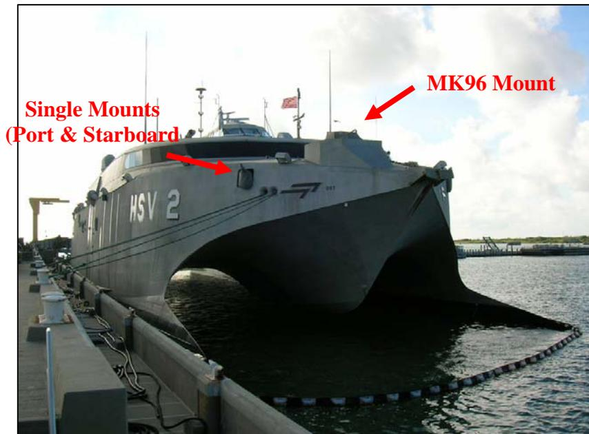
**Figure 2 USS SWIFT Forward Mounts**
