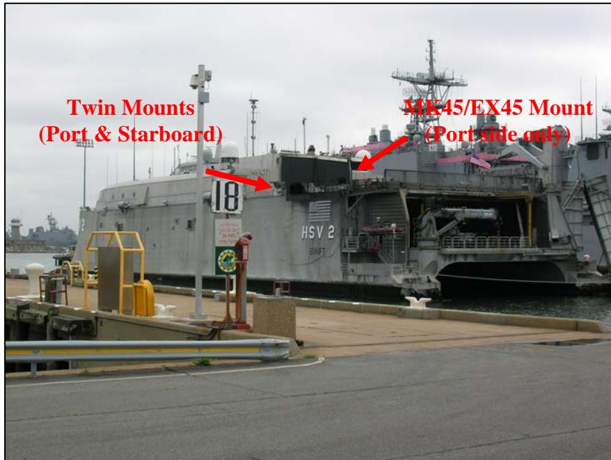
Figure 3 USS SWIFT Flight Deck and Aft Mounts
