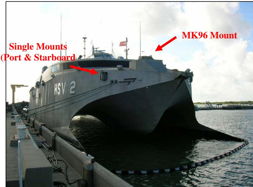
Figure 2 USS SWIFT Forward Mounts
